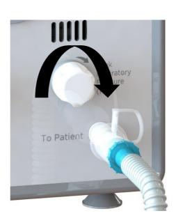
• Close the PEEP head using your thumb and turn the PIP control fully clockwise until the knob no longer rotates.
